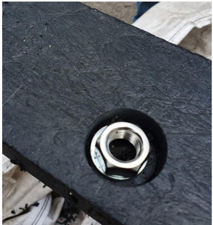
Figure 36: Testing the depth of the drilled hole for the washer and nut.
