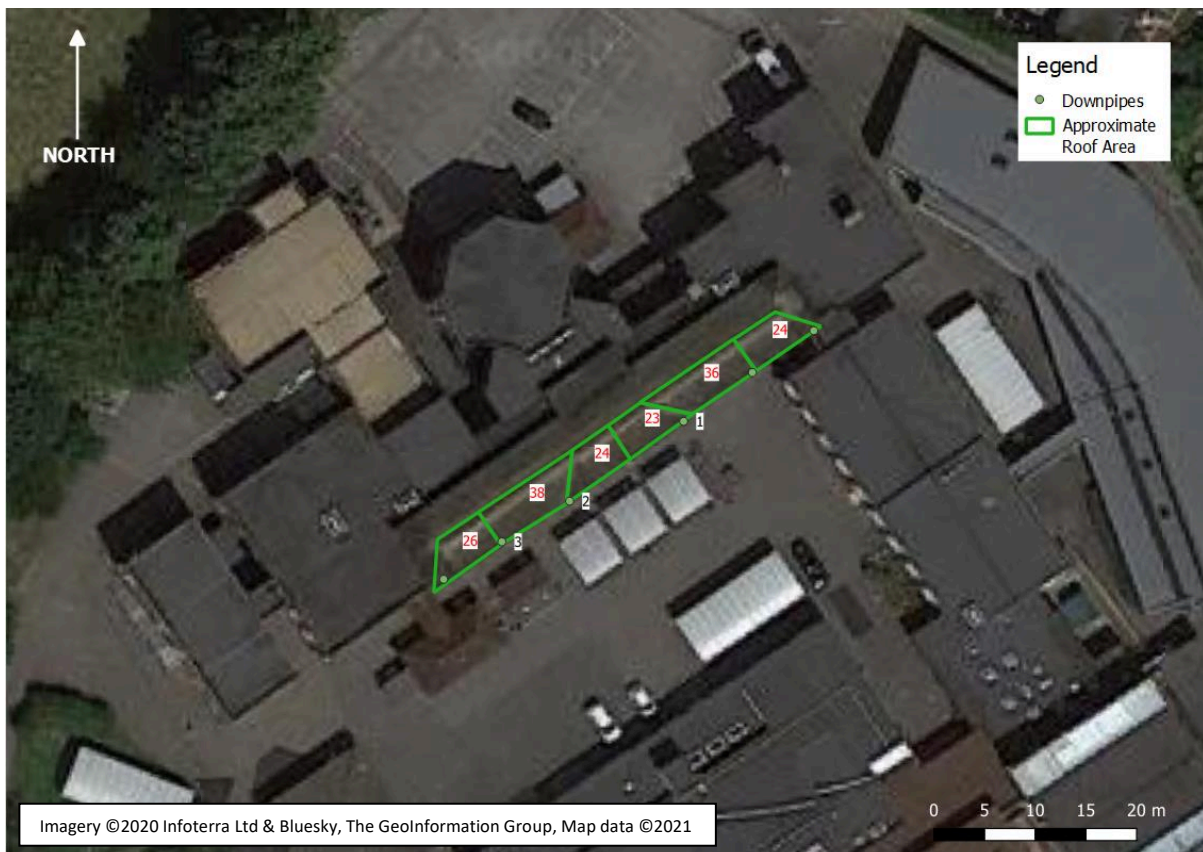
Figure 2. Approximate roof areas and downpipe locations in playground at Carshalton High School for Girls.
