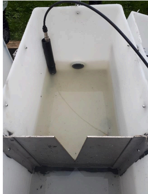
Figure 2. V-notch housed in PVC box. The bottom right image shows the level logger and stilling to record water level.
