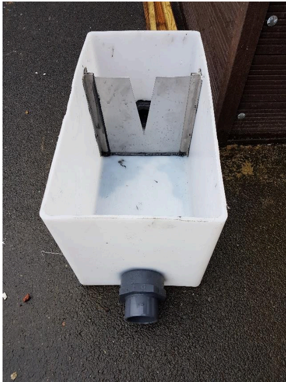
Figure 2. V-notch housed in PVC box. The bottom right image shows the level logger and stilling to record water level.
