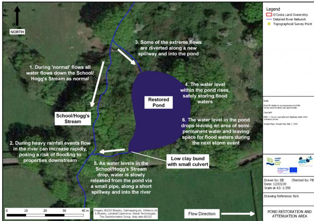
Figure 69. Annotated design for Kingsnoad pond, developed from opportunity mapping and site visits.
